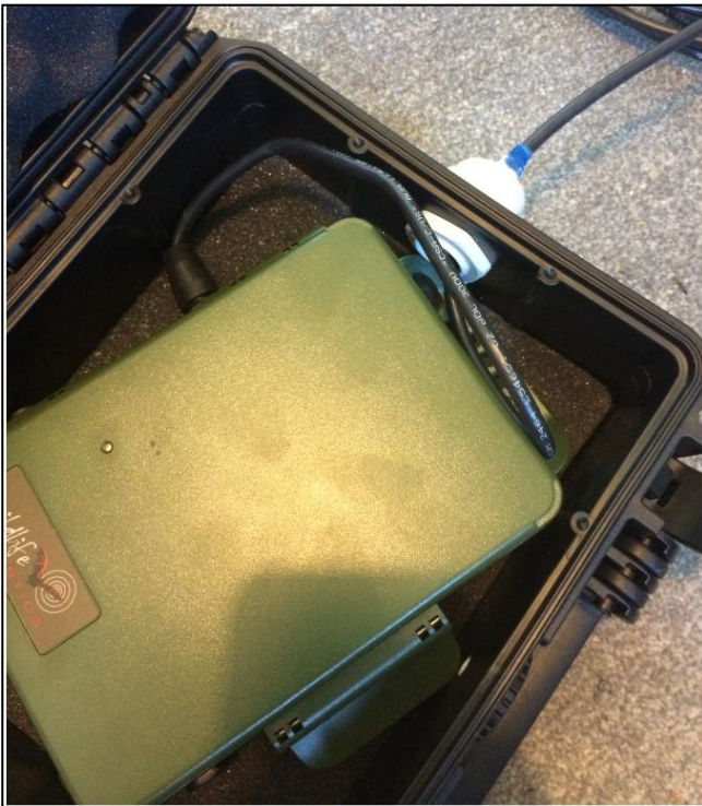
Figure 2-1: Equipment as deployed: Song Meter SM4BAT FS Bat Detector, held within an IP67 armoured case and an SMM-U2 Ultrasonic Microphone.
