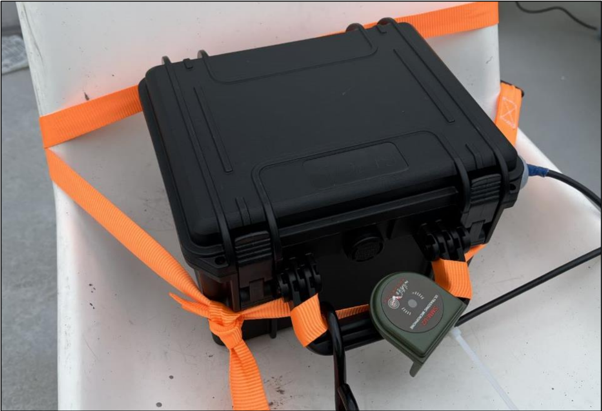
Figure 2-8: MIC: BT02 port side final placement- attached to unit BT07_GPS.
